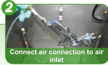
Please ensure that the spray gun is always placed in the correct position inside the washing chamber of self-contained washing machines. **Make sure that no cleaning agent penetrates the air passages of the spray gun.**
