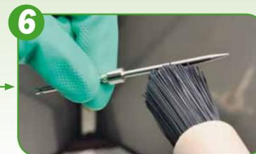
Please make sure that all brushes being used **have no protruding metal wires** as these may damage the spray gun. Please exclusively use recommended tools for cleaning only.
